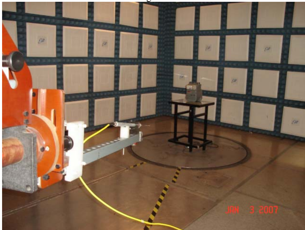
Test Set-up for Radiated Emissions, 916.45MHz Horizontal Polarization
