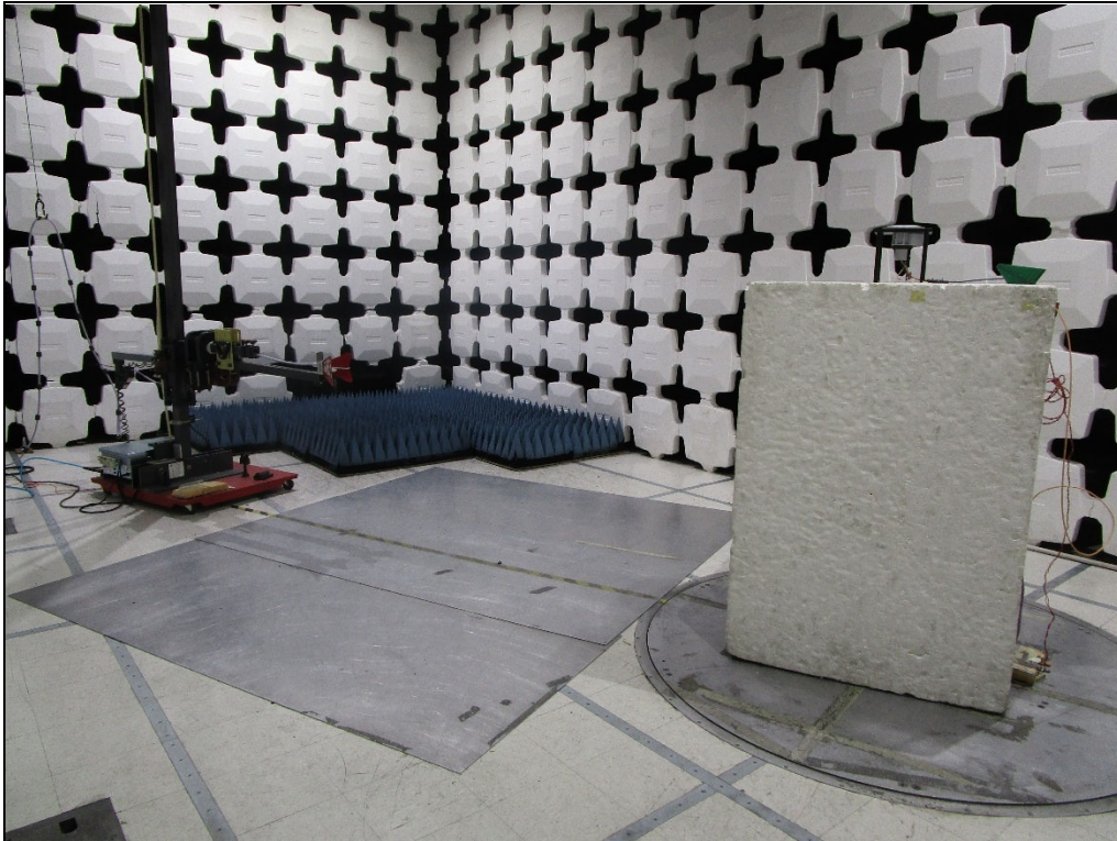
Test Setup for Spurious Emissions: Horizontal Polarization
