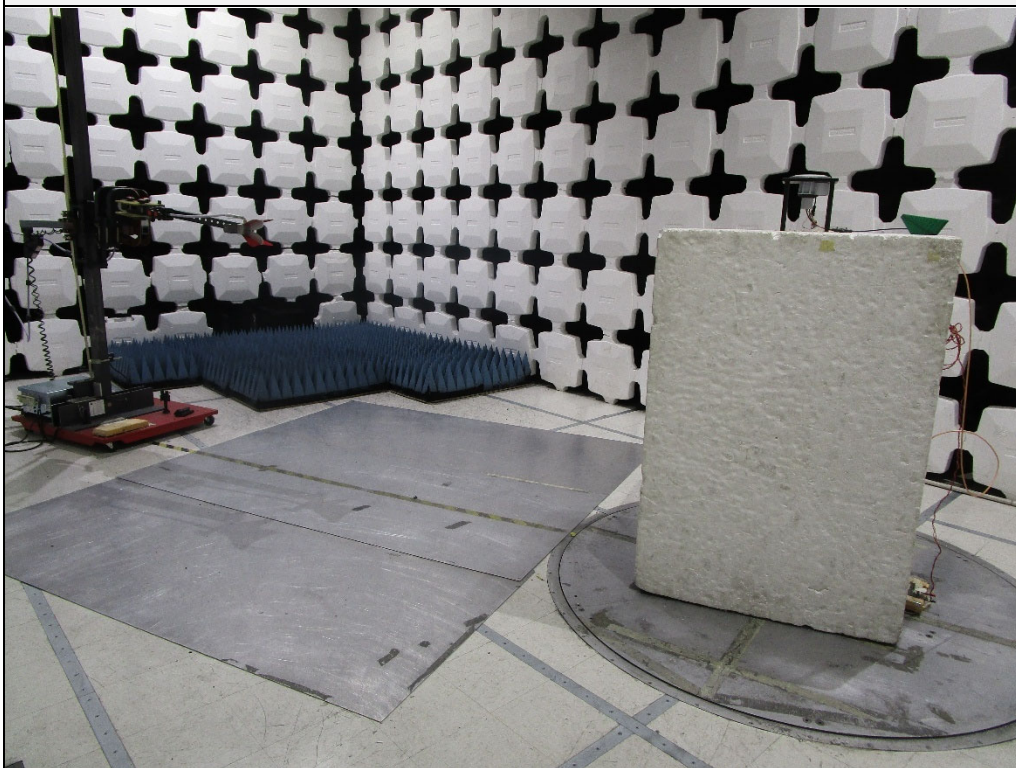
Test Setup for Spurious Emissions: Vertical Polarization
