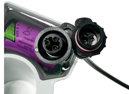
Figure 2: 3-socket Twist Tight connector with black cable
