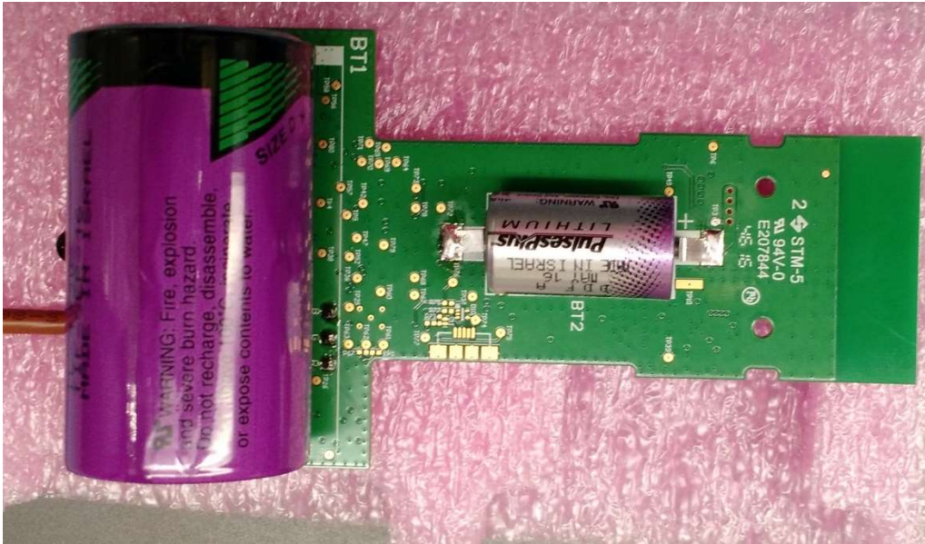
Figure 3 Batteries installed on PCBA.
