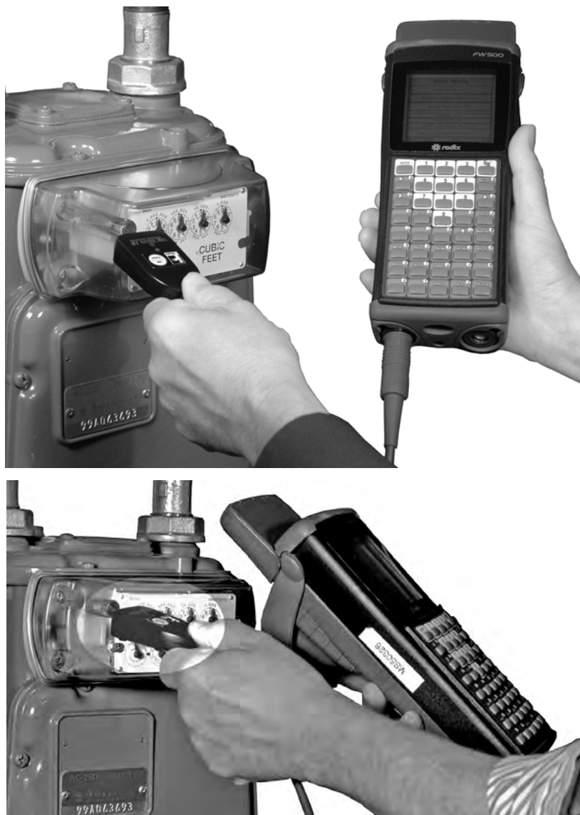
Figure 30: Align with IR Cable
