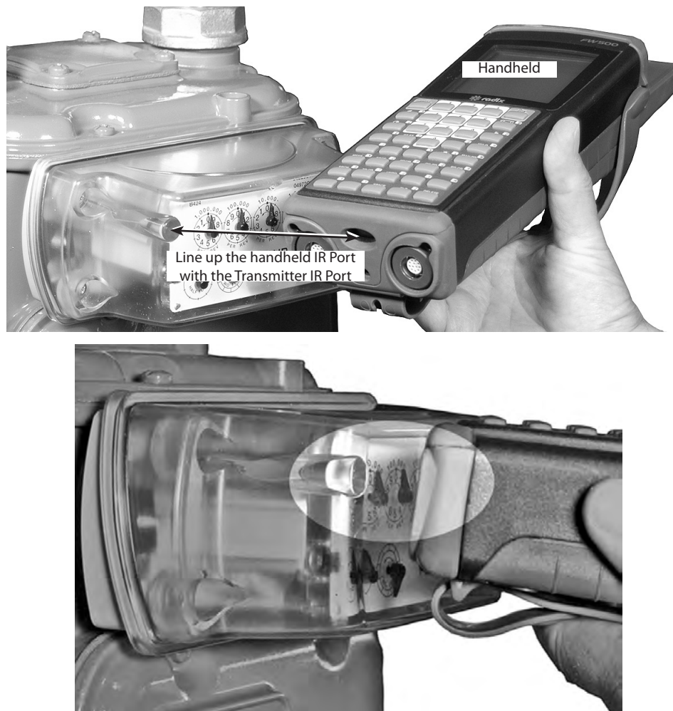
Figure 29: Align IR Ports
