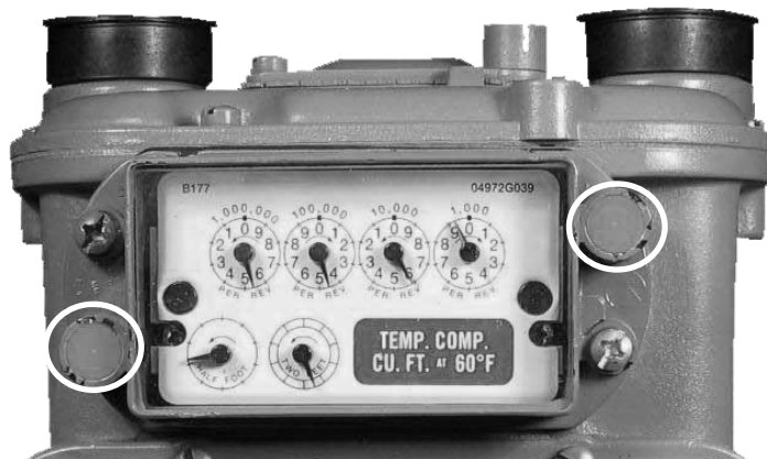
Figure 2: Tamper Plugs (circled)
