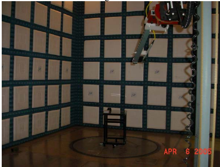
TEST SETUP FOR MEASUREMENT OF RADIATED EMISSIONS, VERTICAL POLARIZATION
