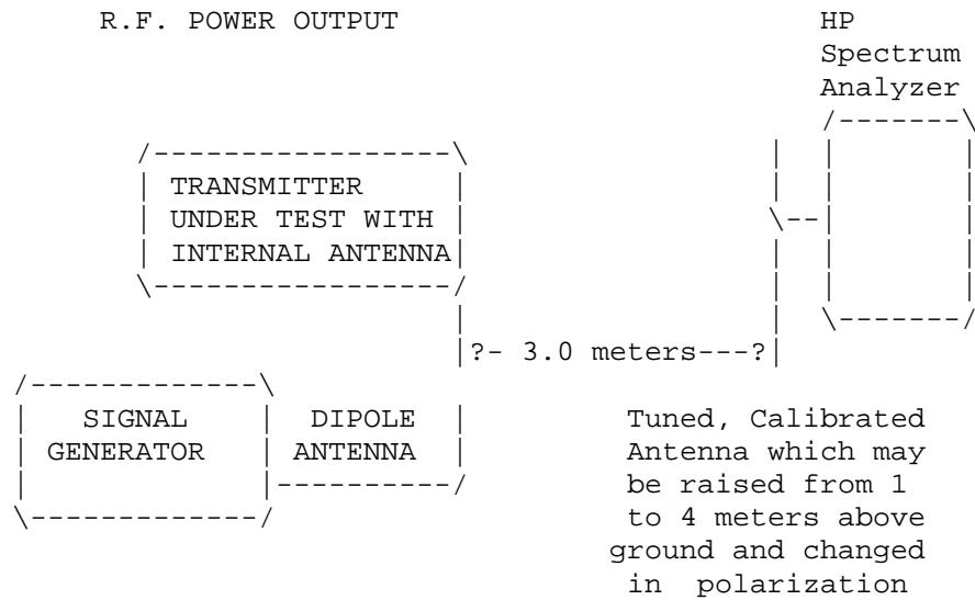
Equipment placed 1 meter above ground on a rotatable platform. The center of the Dipole antenna at the center of the platform and the output of the signal generator adjusted to produce the same meter reading as measured for the fundamental in the radiated emissions test.
