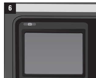
6 Red LED begins to flicker and the screen enters sleep mode. The system is now armed and the tools are secured
