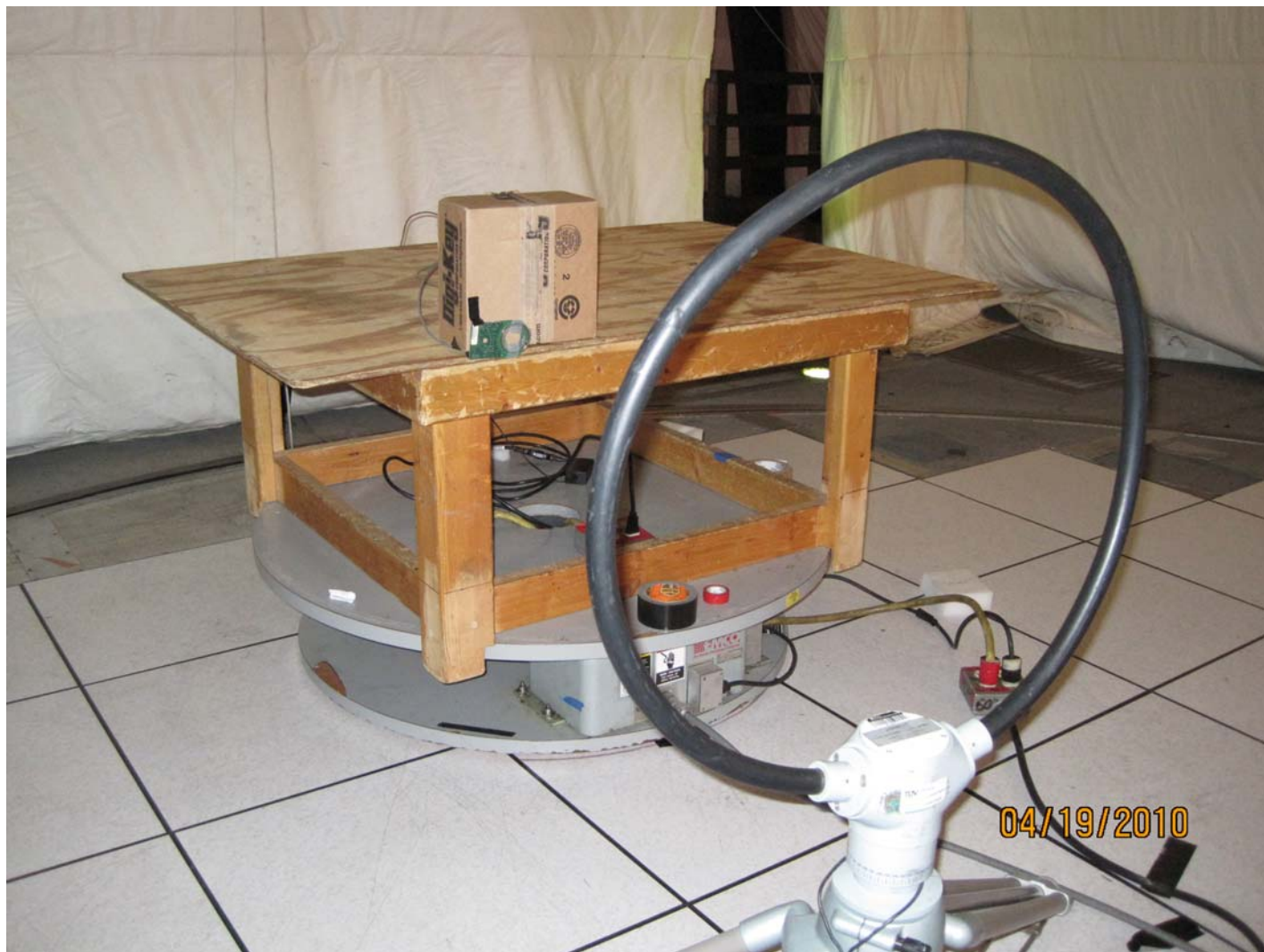
Test-setup photo(s): General Field Strength Limits 0.009 – 30 MHz
