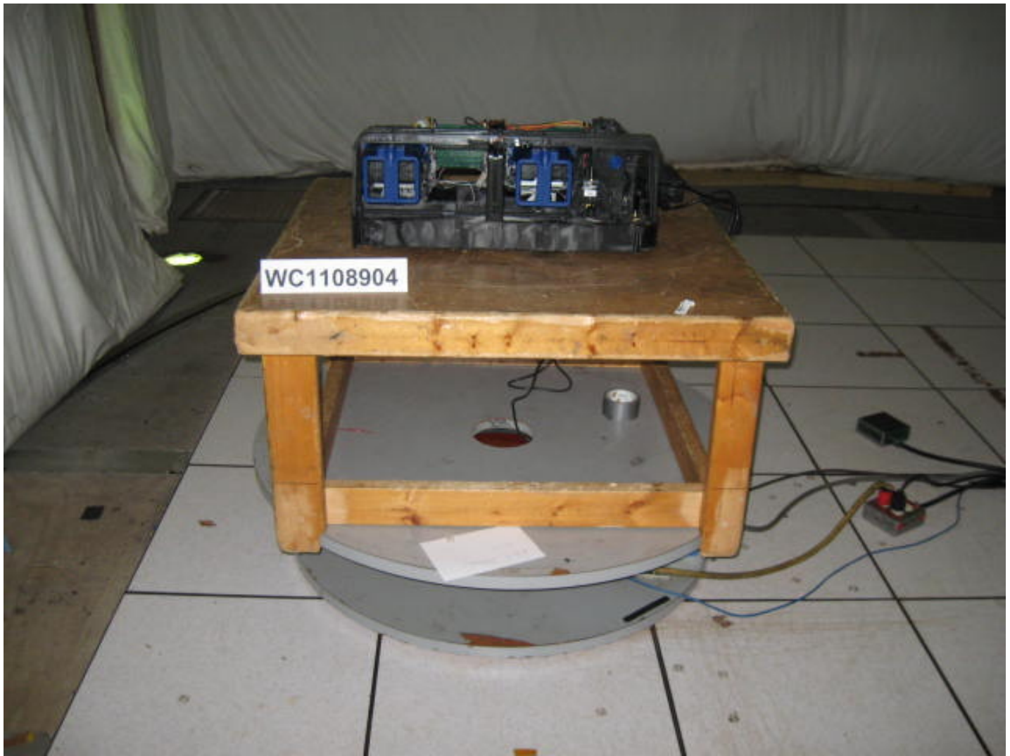
Test-setup photo(s): Radiated Emissions 30 - 1000 MHz
