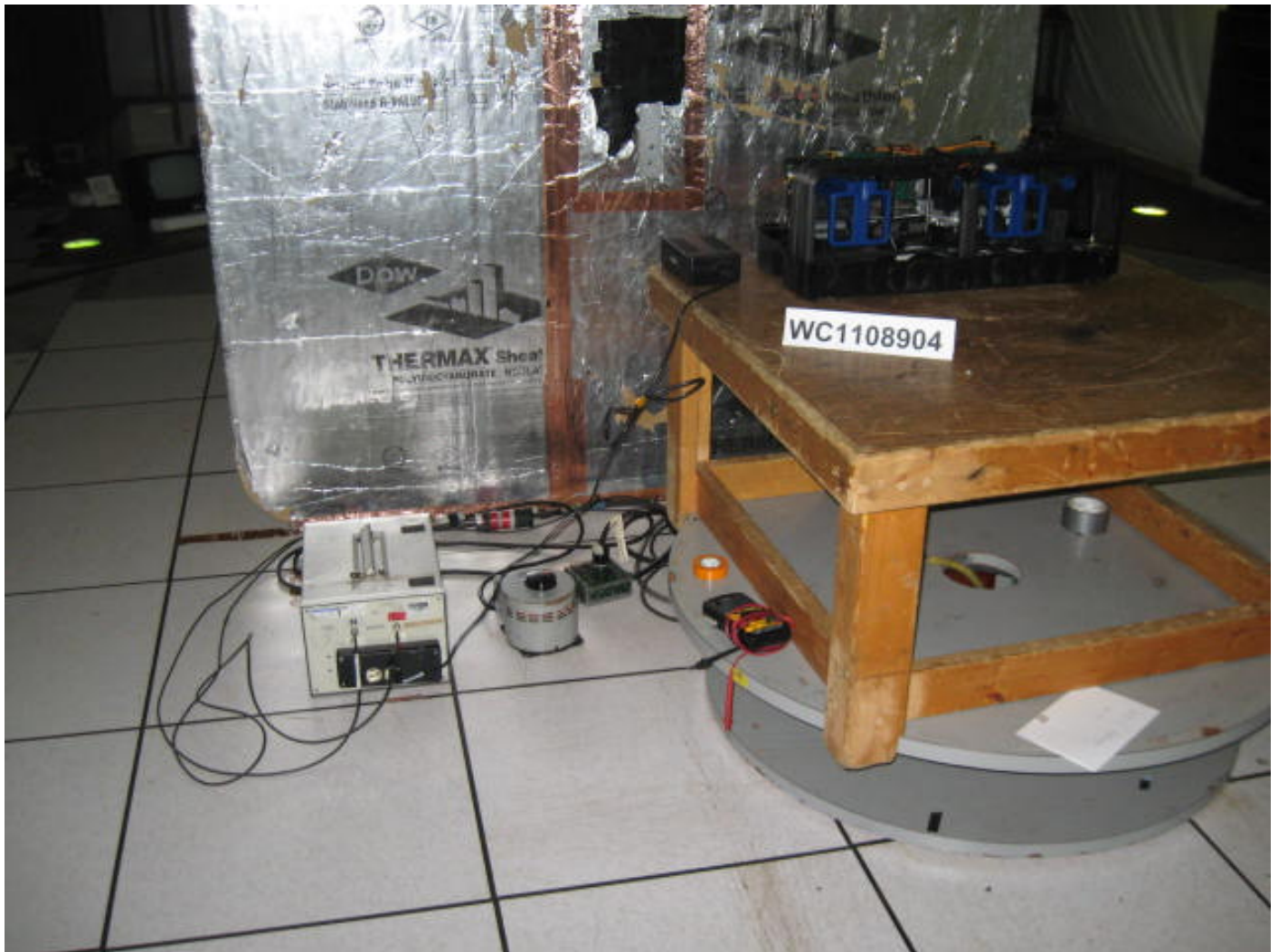
Test-setup photo(s): Conducted Emissions, AC lines, 150 kHz - 30 MHz
