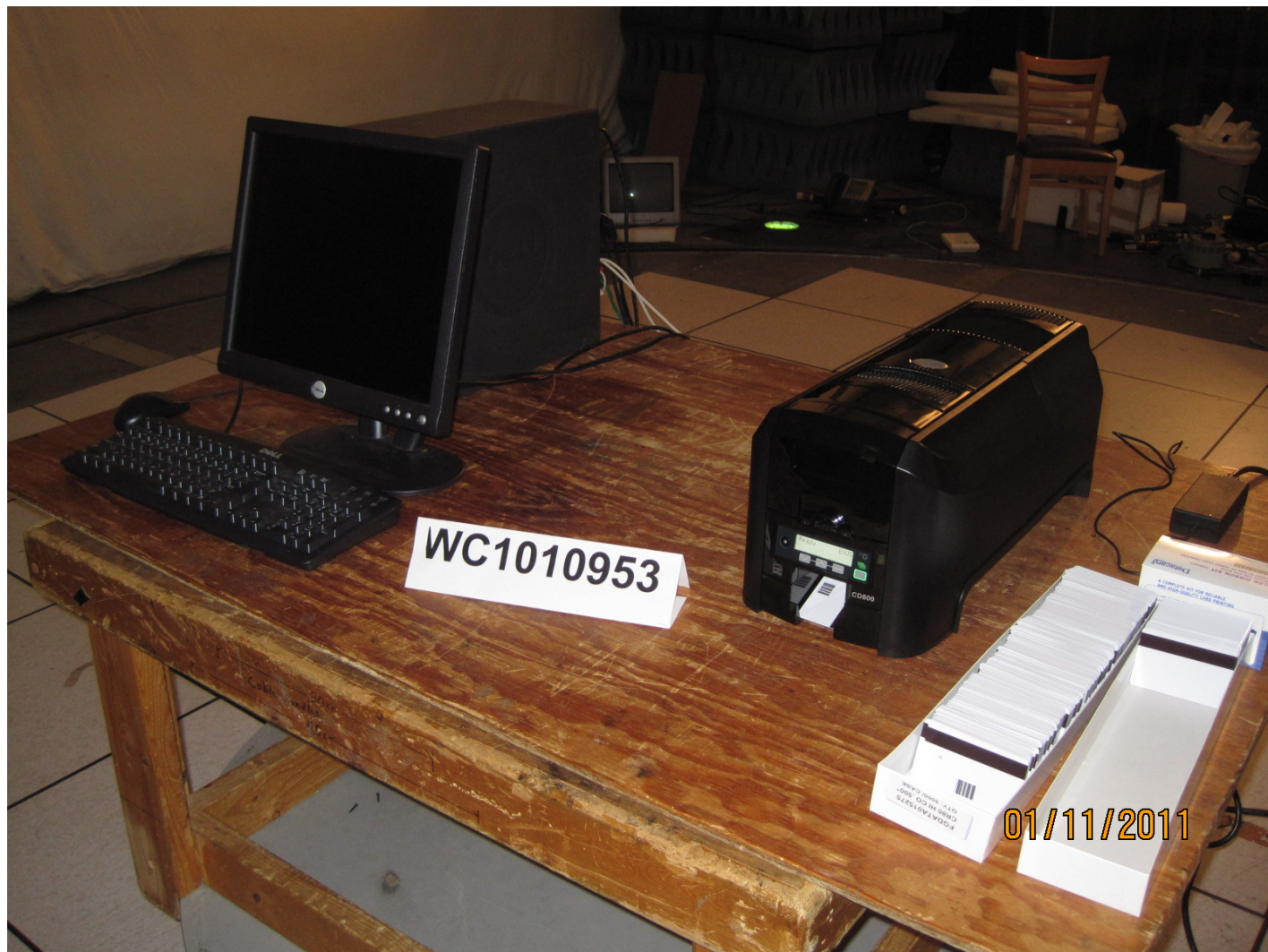
Test-setup photo(s): Radiated Emissions 30 - 1000 MHz
