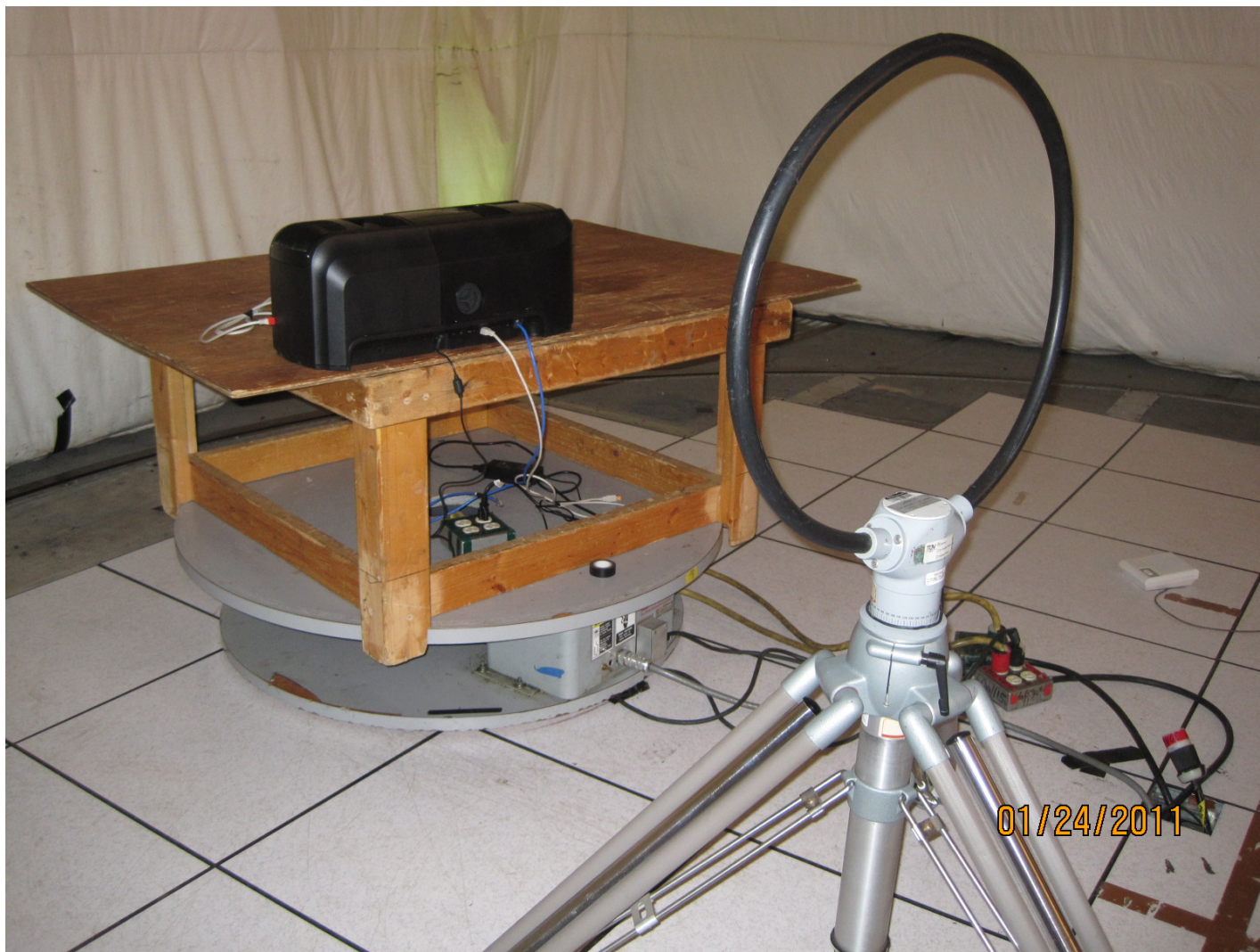
Test-setup photo(s): General Field Strength Limits 0.009 – 30 MHz
