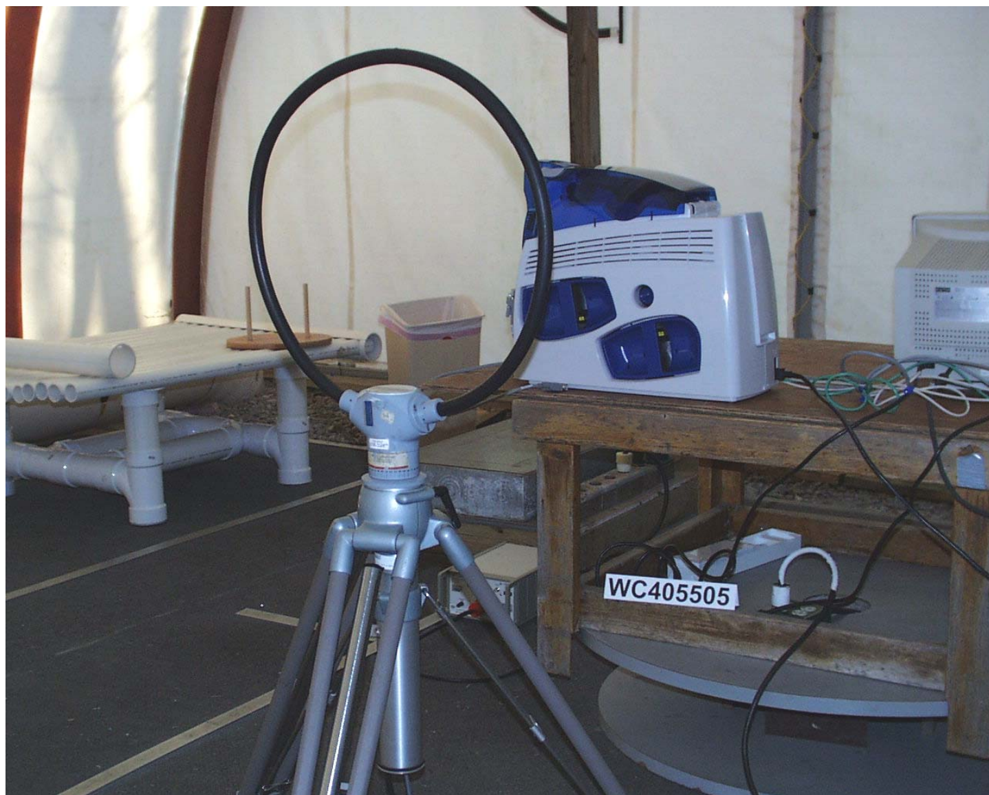
Test-setup photo(s): Radiated emission 10 kHz - 30 MHz
