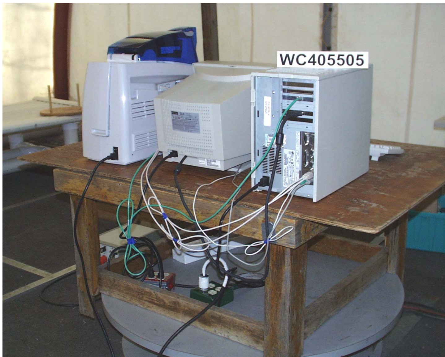
Test-setup photo(s): Radiated emission 30 MHz - 1000 MHz
