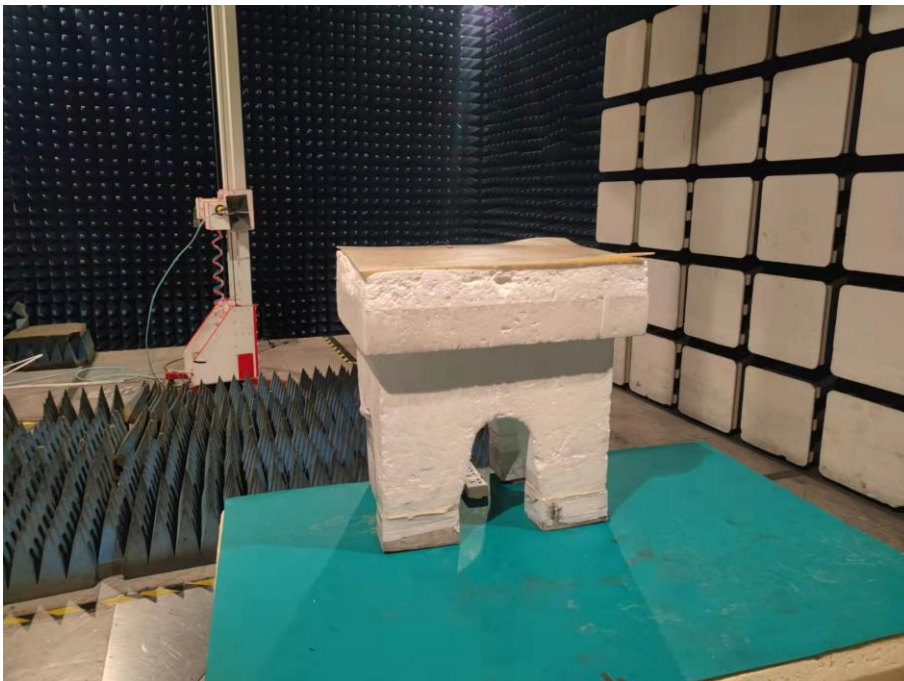
Spurious Emission Test Setup (Above 1GHz)
