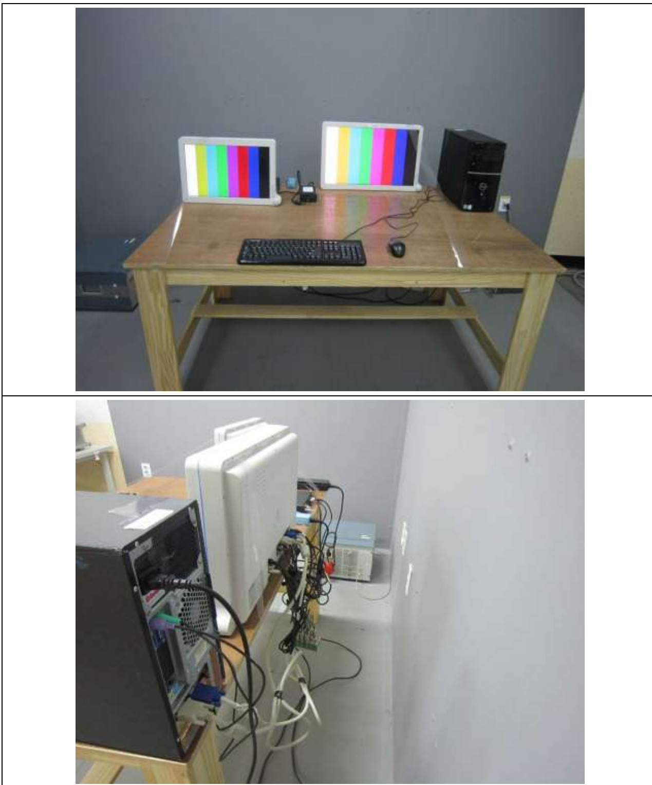
Figure 2. Conducted Emission Test Setup: SDI Mode
