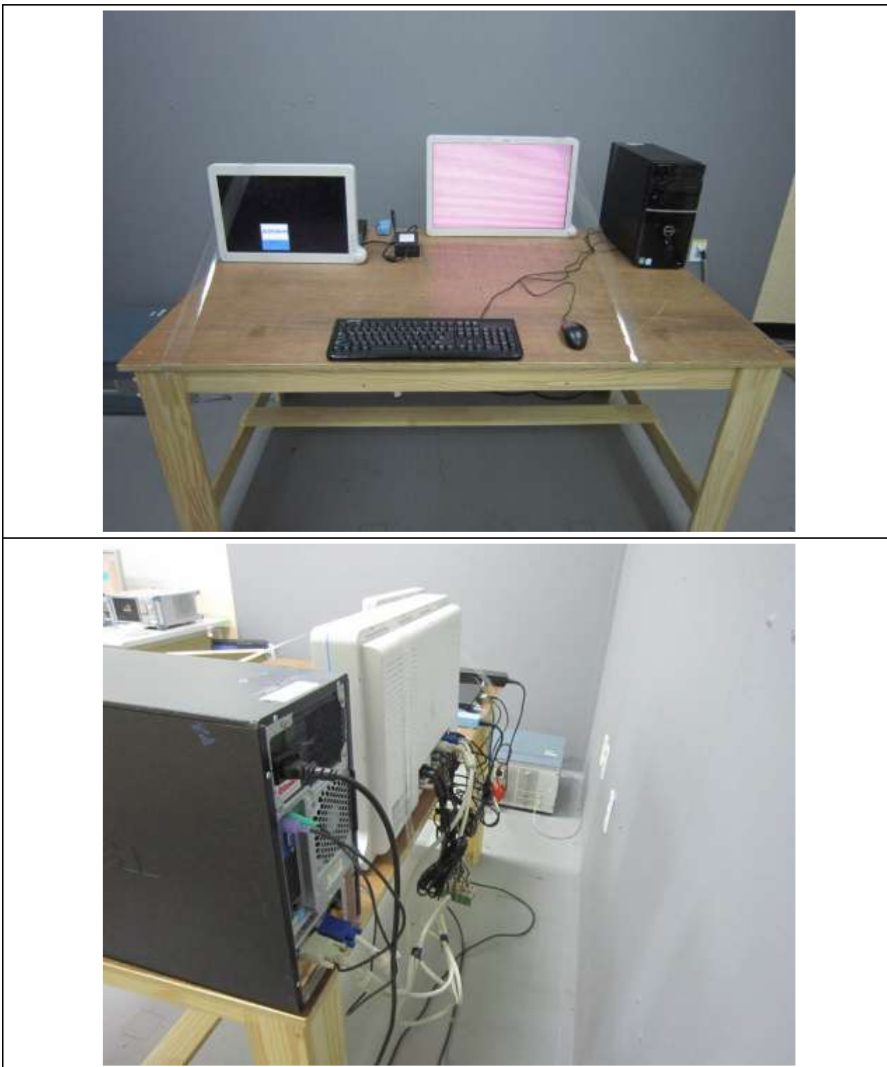
Figure 1. Conducted Emission Test Setup: DVI Mode
