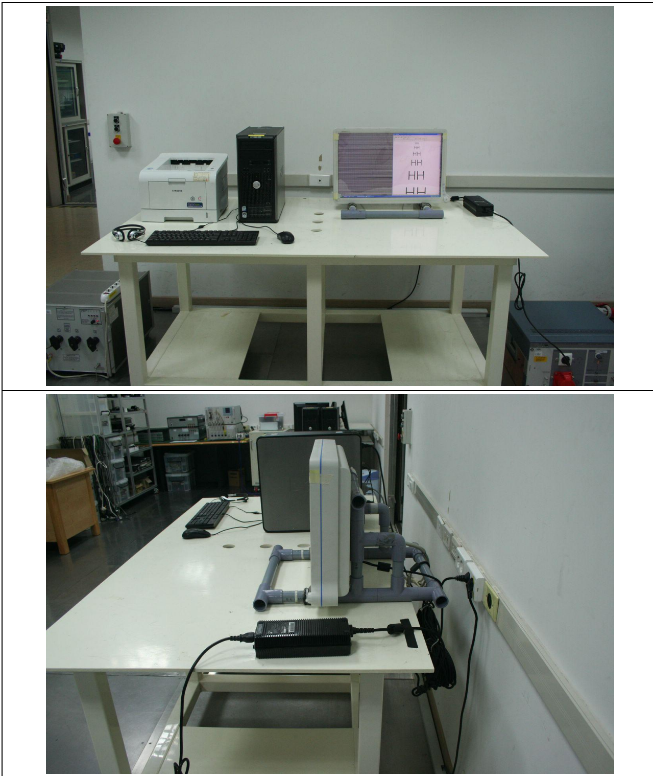
Figure 1. Conducted Emission Test Setup for DVI Mode:
