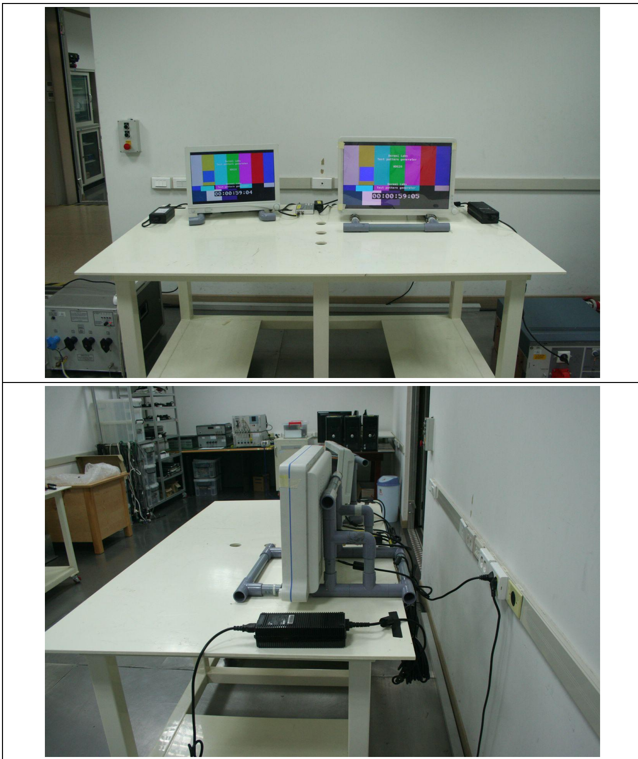
Figure 4. Conducted Emission Test Setup for SDI In/Out Mode:
