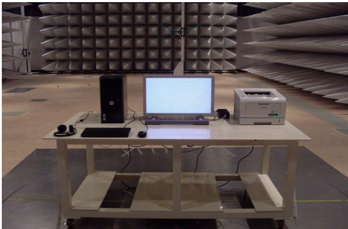
Figure 13, Radiated emission test setup for Test Configuration 2
