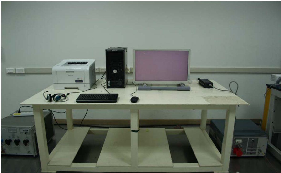
Figure 1. Conducted Emission Test Setup for Test Configuration 1
