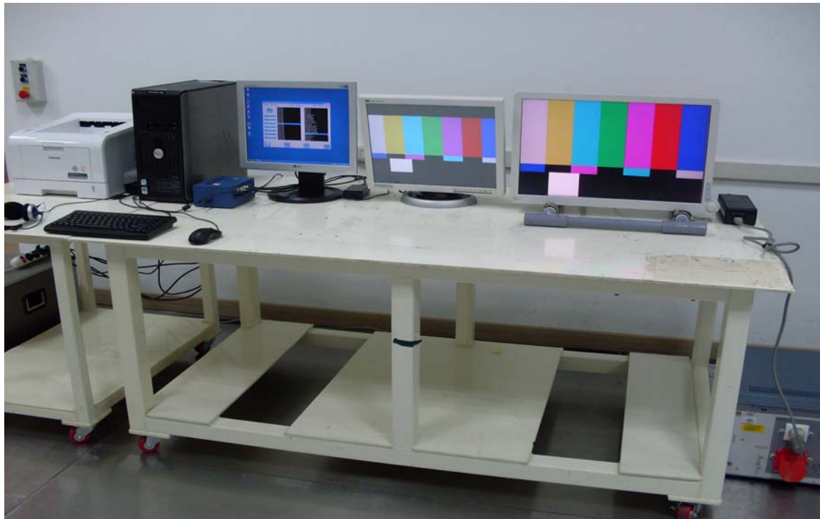
Figure 3. Conducted Emission Test Setup for Test Configuration 1
