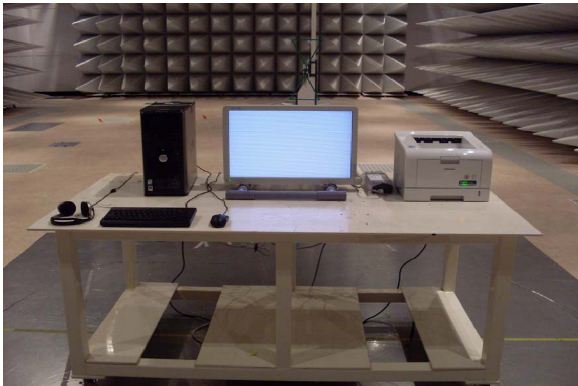
Figure 9, Radiated emission test setup for Test Configuration 1
