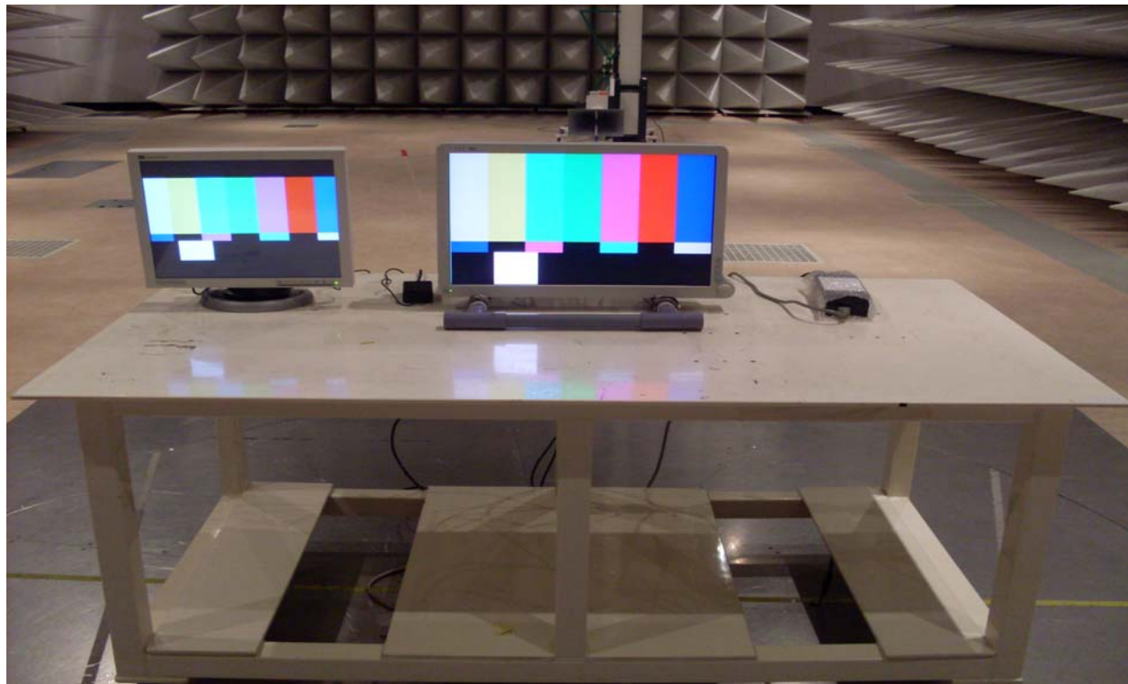
Figure 9, Radiated emission test setup for Test Configuration 1
