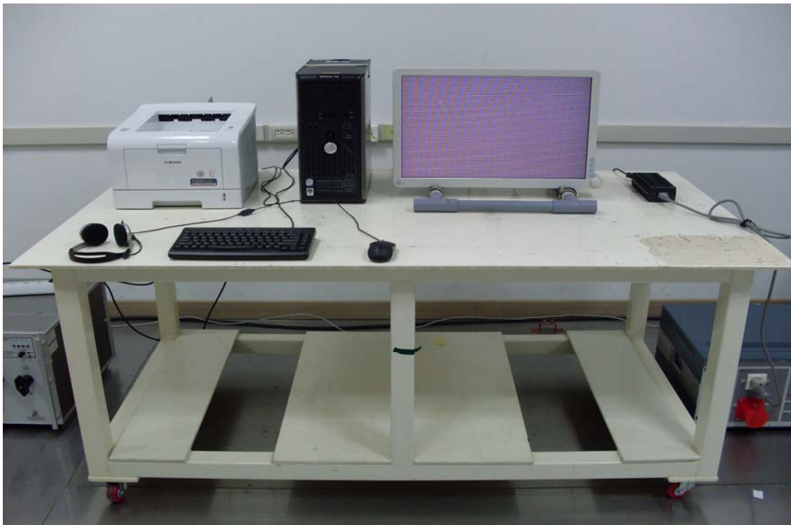
Figure 5. Conducted Emission Test Setup for Test Configuration 2
