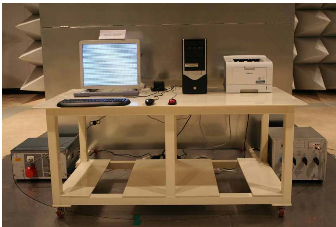
Figure 1 Conducted Emission Test Setup: DVI Mode (LCD Panel: TX54D31VC0CAB)
