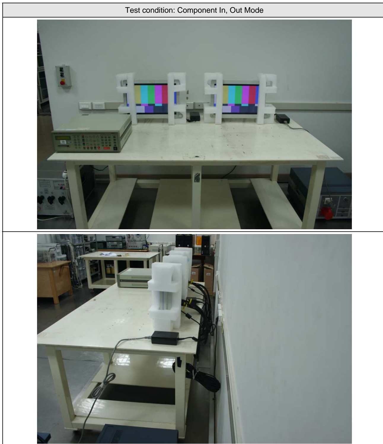
Figure 2. Conducted Emission Test Setup Test
