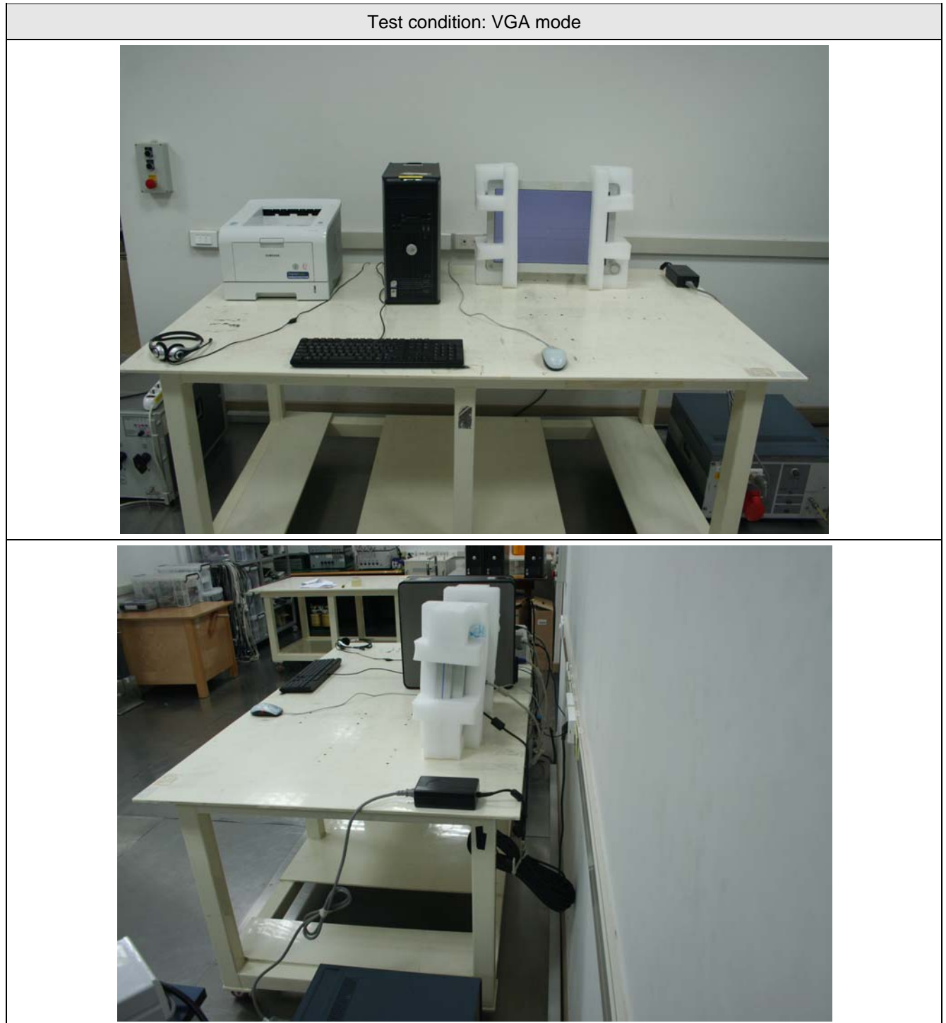
Figure 1. Conducted Emission Test Setup
