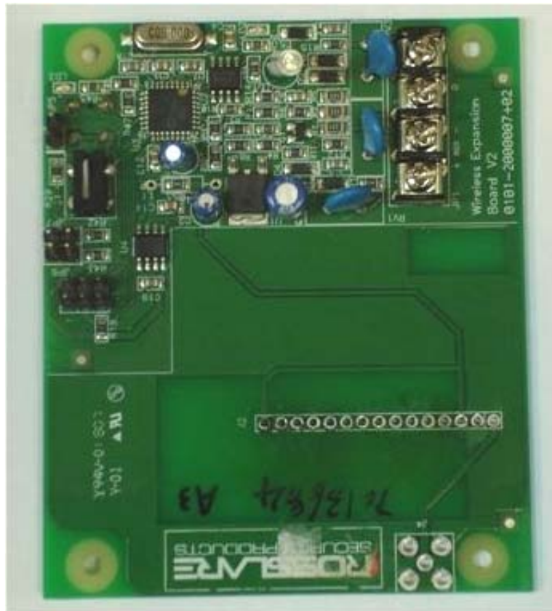
Photograph No.6 XR-16AG main PCB with daughter PCBs removed
