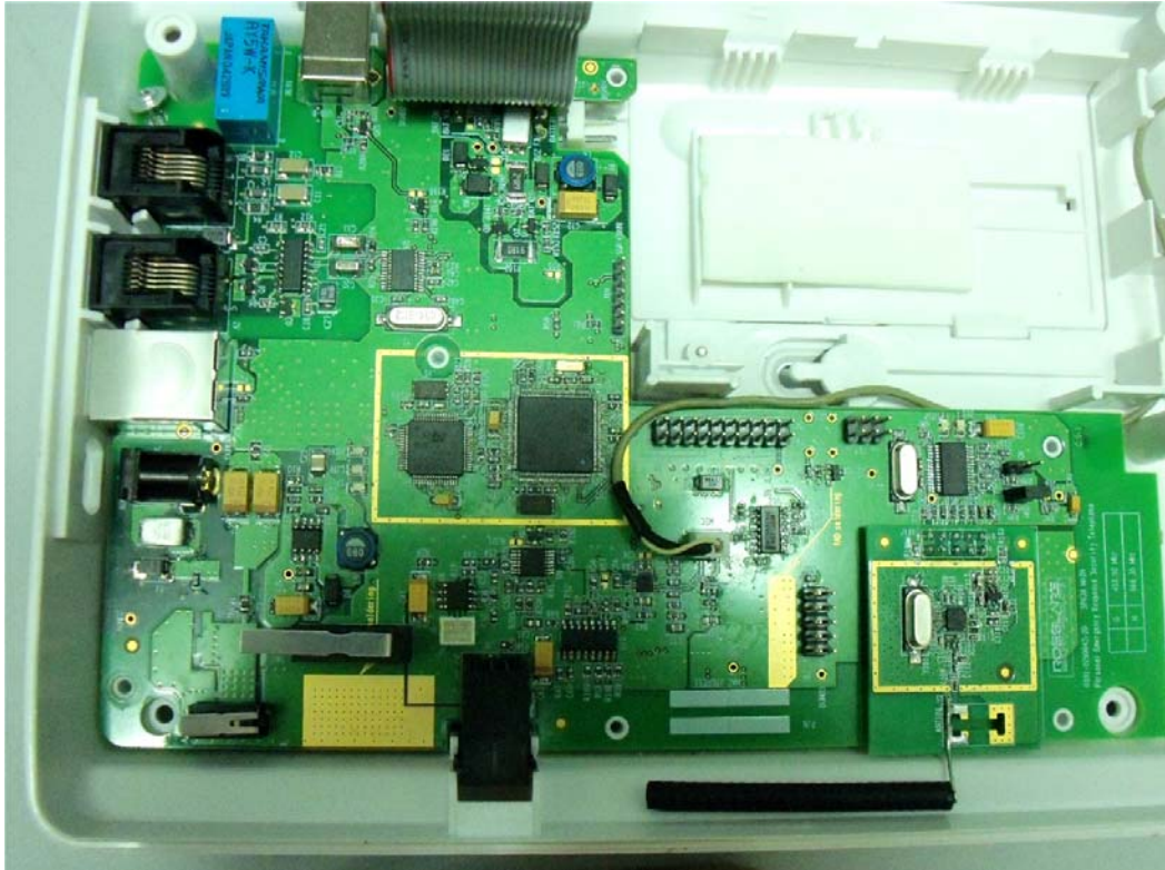
Photograph No.3 Wireless Elderly Assist SP-03V2G internal view without battery
