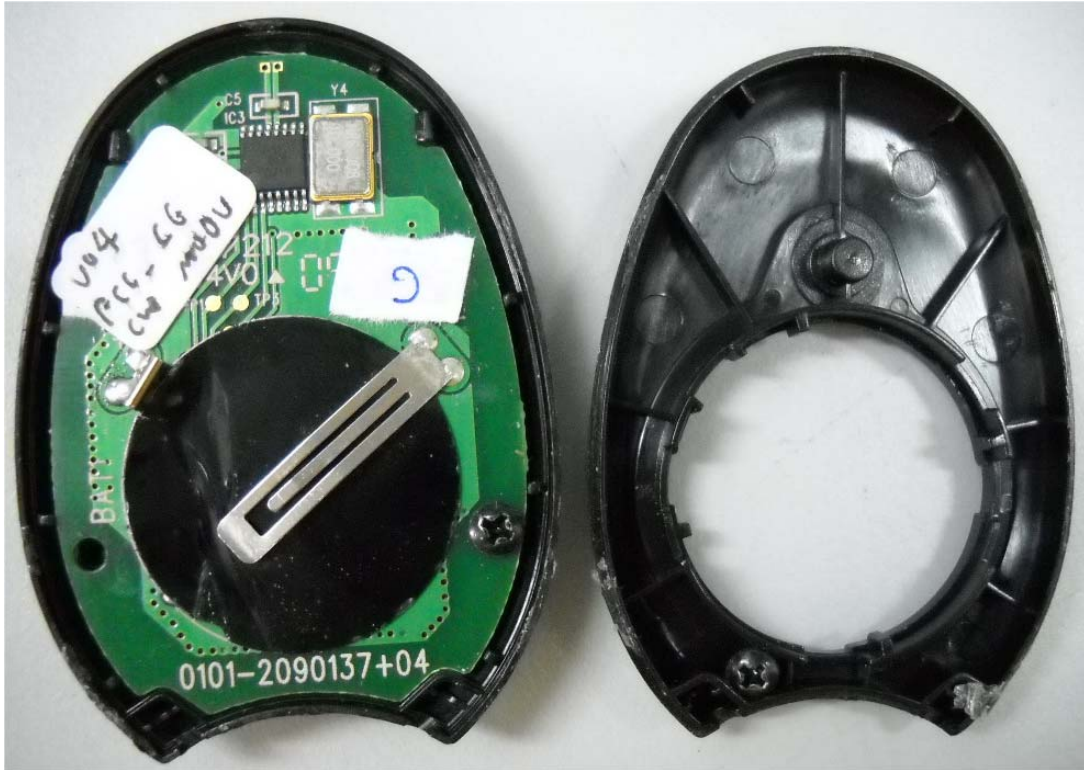
Photograph No.3 SA-33G remote control internal view
