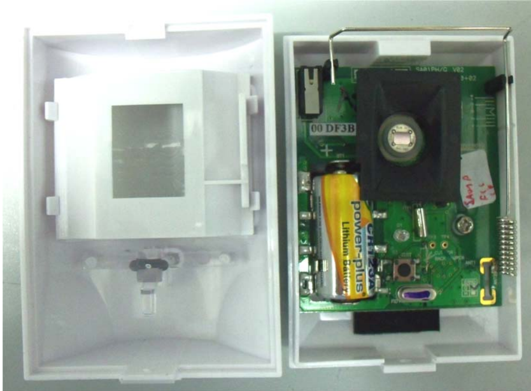
Photograph No.1 SA-01PG PIR detector internal view
