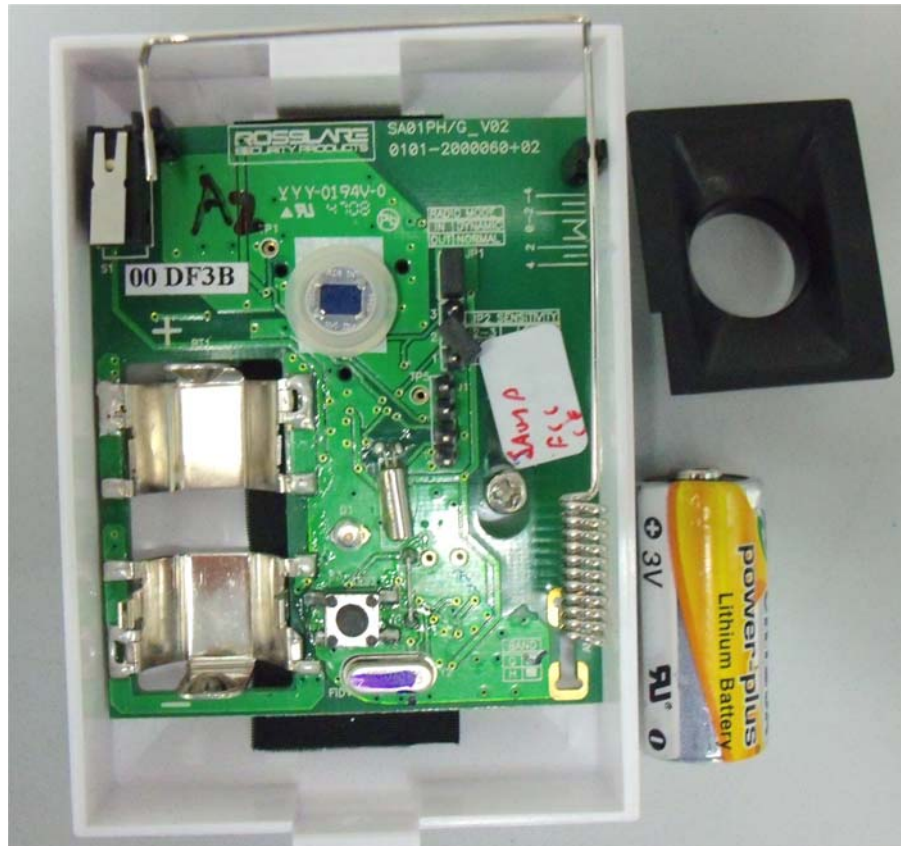
Photograph No.2 SA-01PG PIR detector internal view
