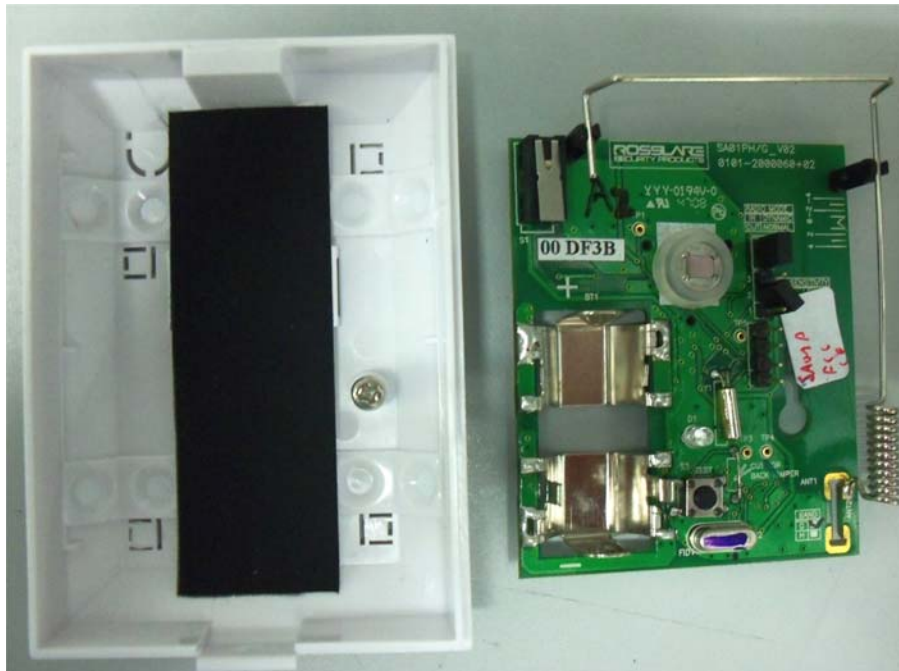
Photograph No.3 SA-01PG PIR detector internal view
