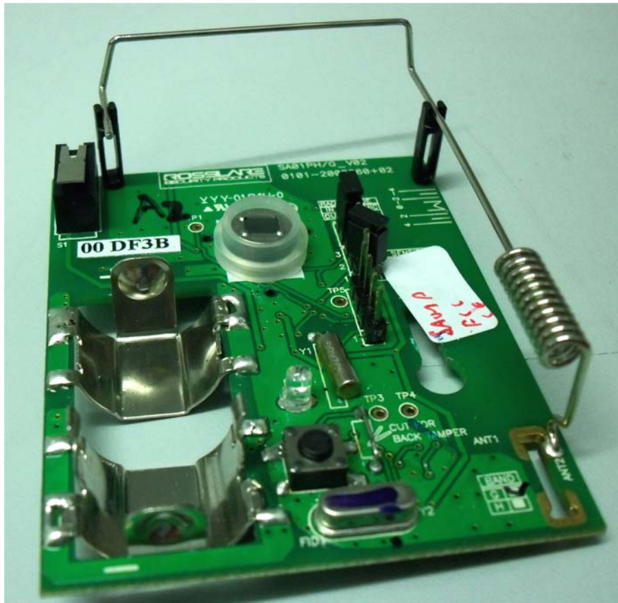
Photograph No.6 Antenna close view
