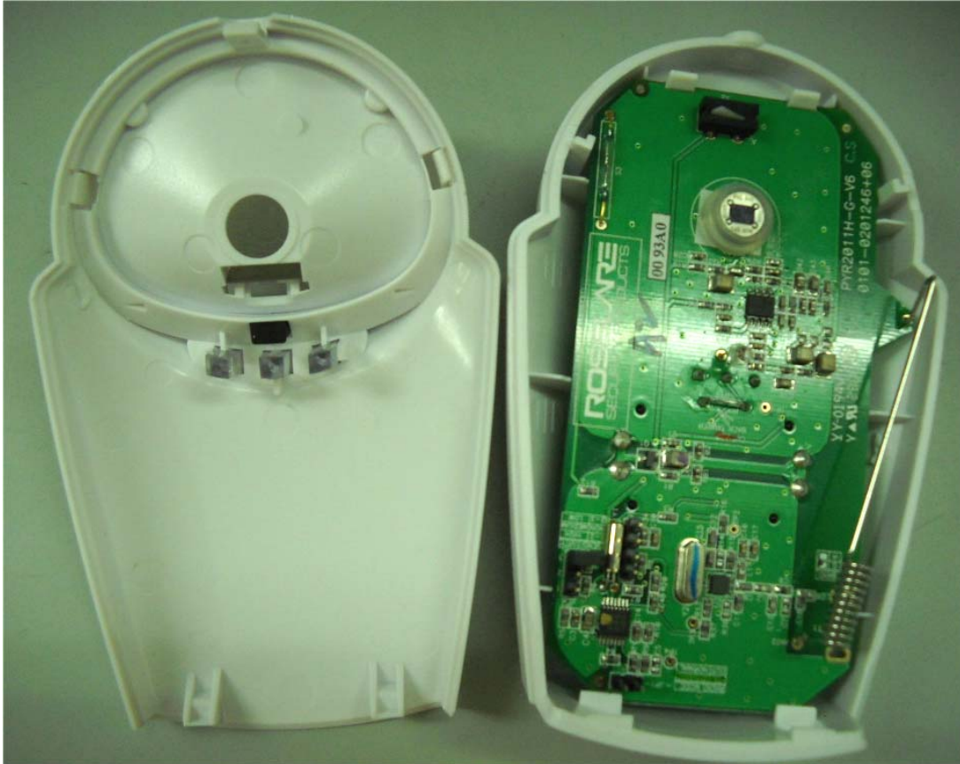
Photograph No.1 PYR-2011AG detector internal view
