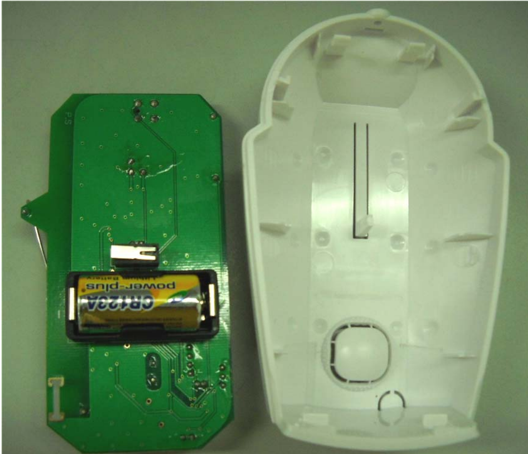
Photograph No.2 PYR-2011AG detector internal view
