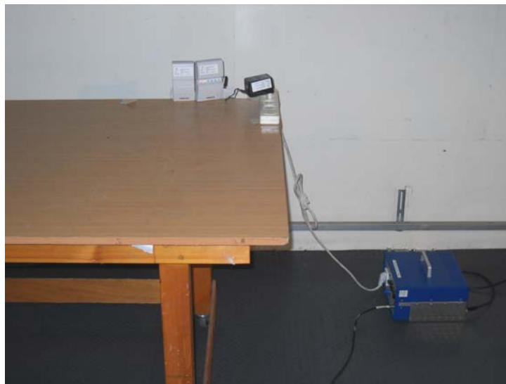
Photograph 8.1.1 Setup for conducted emission measurements
