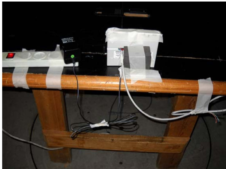
Photograph 8.2.2 Setup for radiated emission measurements, EUT cabling
