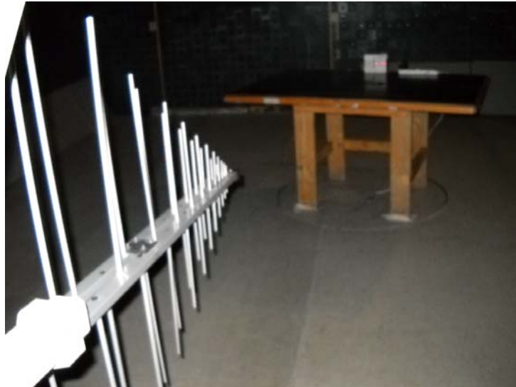
Photograph 8.2.2 Setup for radiated emission measurements, EUT cabling
