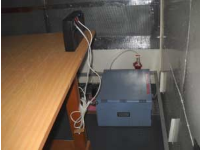
Photograph No.7 Setup for conducted emission measurements on the power lines
