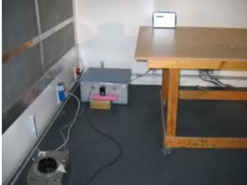
Photograph No.6 Setup for conducted emission measurements on the power lines
