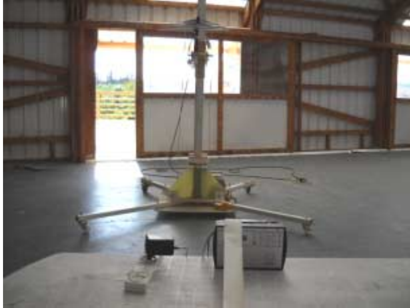
Photograph No.5 Setup for spurious emission measurements at the OATS, EUT close view
