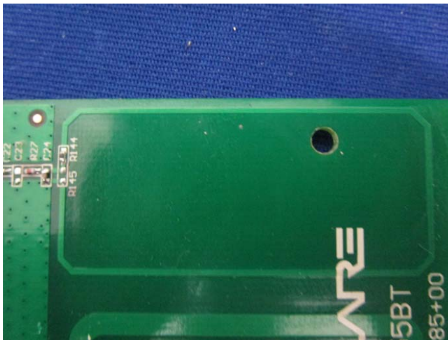
EUT – 915MHz Module Antenna View
