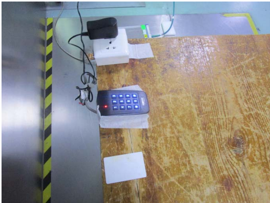
Conducted Emissions – Side View
