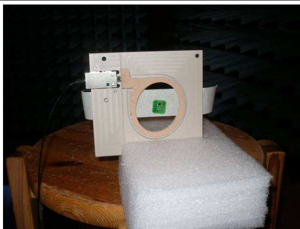
EUT antenna with lens simulation print in the center
