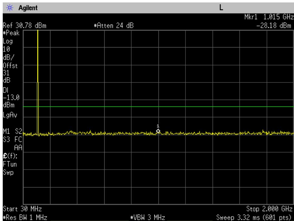
30 MHz-2GHz Low Channel Conducted Spurious Emissions
