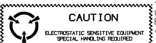
THIS ASSEMBLY INCLUDES COMPONENTS WHICH ARE SUBJECT TO DAMAGE BY ELECTROSTATIC CHARGES: THEREFORE, ALL COMPONENTS SHALL BE HANDLED IN ACCORDANCE WITH GUIDELINES FOR ELECTROSTATIC DISCHARGE CONTROL.
