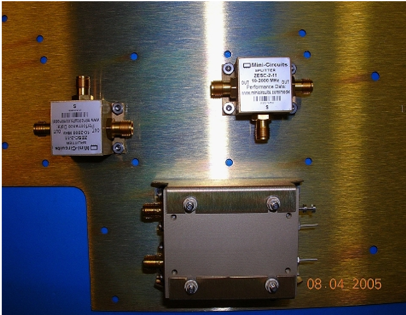
Figure 9: 1252-F-0017 2 splitters and 10MHz OCXO Installed
