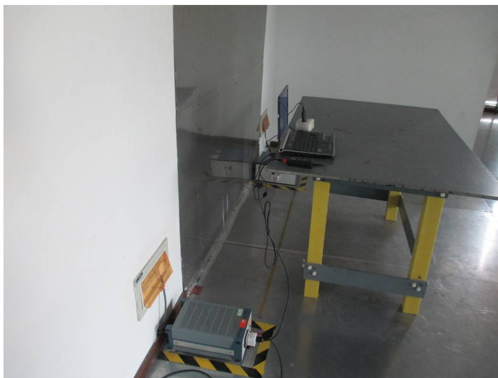
Conducted Emissions Test Setup Side View
