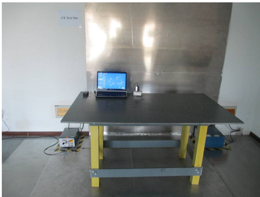
Conducted Emissions Test Setup Front View
