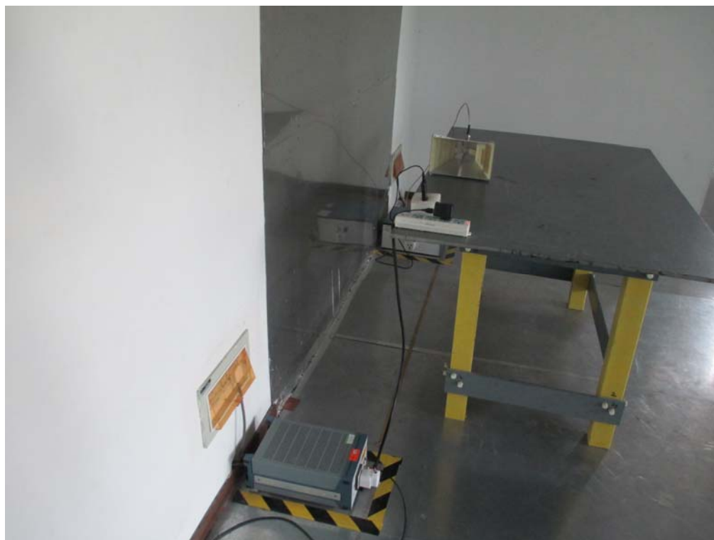
Conducted Emissions Test Setup Side View
