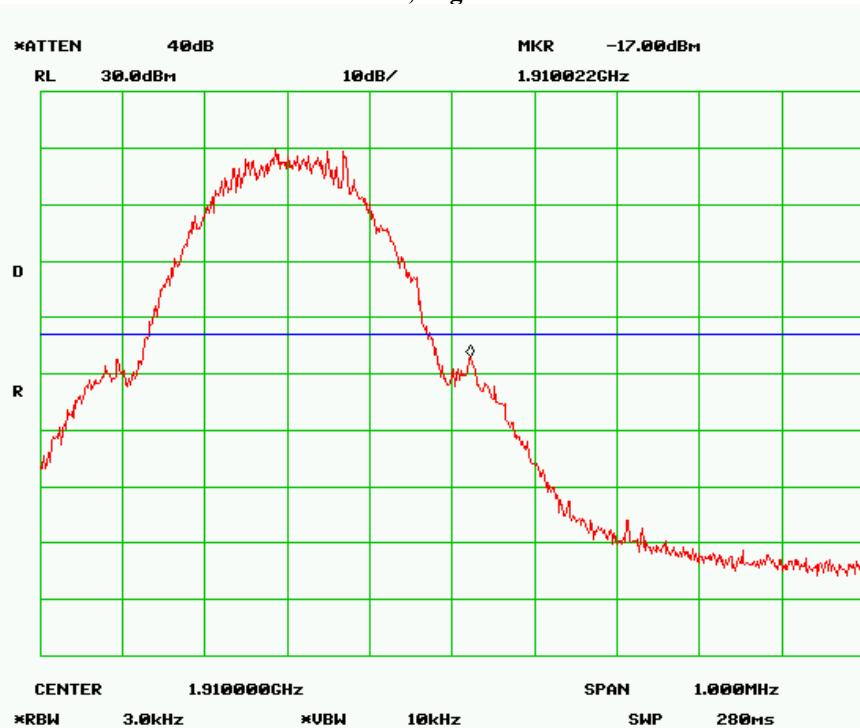
Note: offset= cable loss + 10log(1%\*26dB/3kHz)
