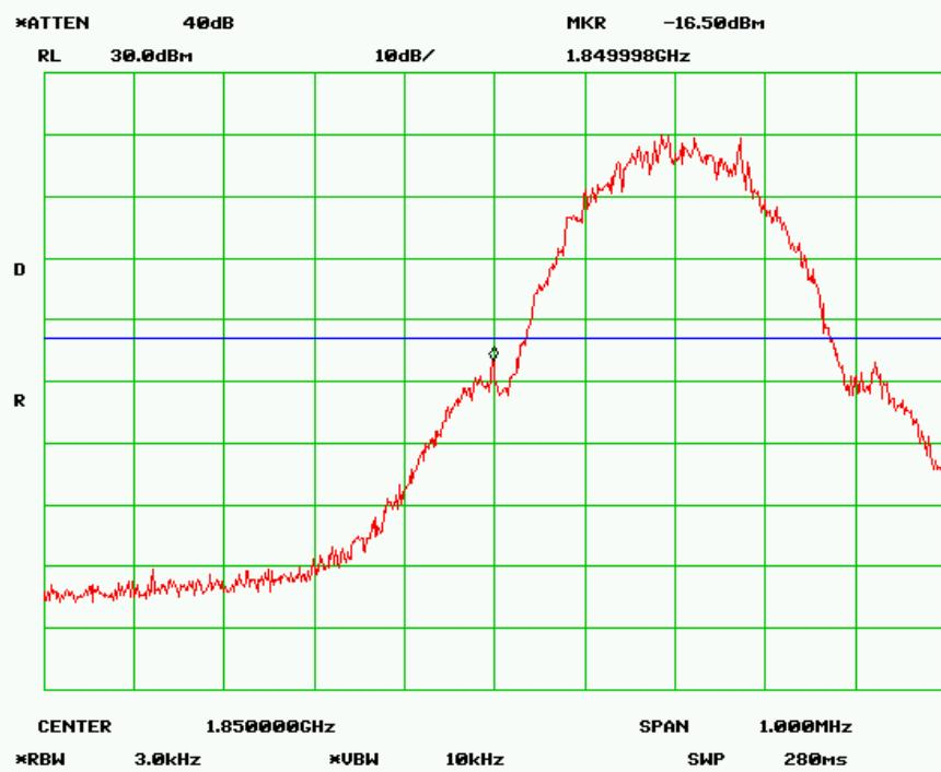
Note: offset= cable loss + 10log(1%\*26dB/3kHz)
