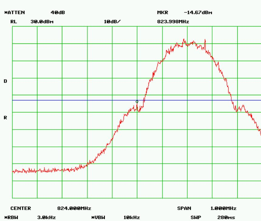
Note: offset= cable loss + 10log(1%\*26dB/3kHz)
