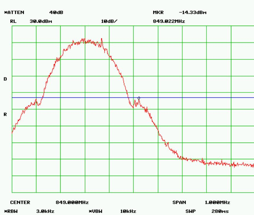
Note: offset= cable loss + 10log(1%\*26dB/3kHz)
