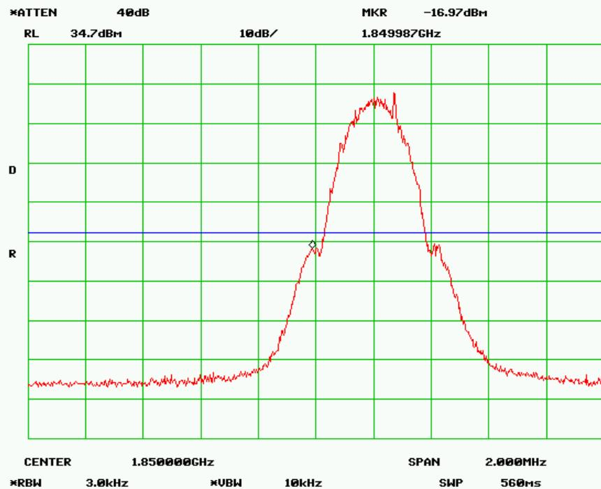
Note: offset= cable loss + 10log(1%\*26dB/3kHz)
