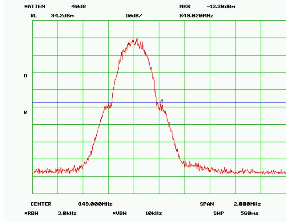
Note: offset= cable loss + 10log(1%\*26dB/3kHz)
