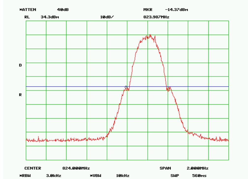
Note: offset= cable loss + 10log(1%\*26dB/3kHz)
