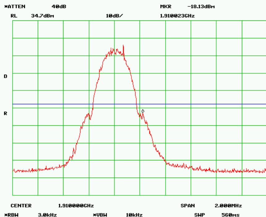
Note: offset= cable loss + 10log(1%\*26dB/3kHz)
