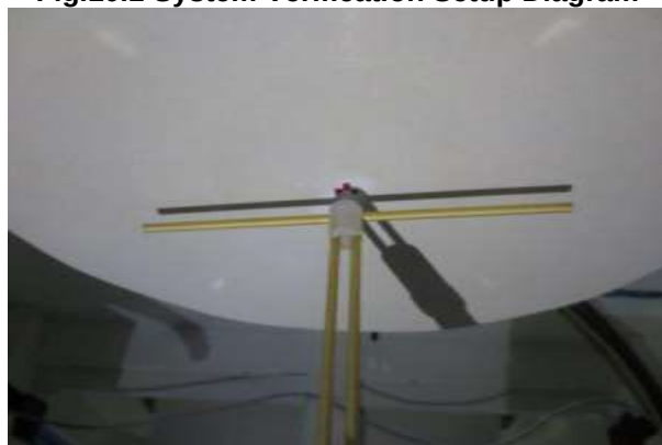
Fig.10.2 Photo of Dipole setup
