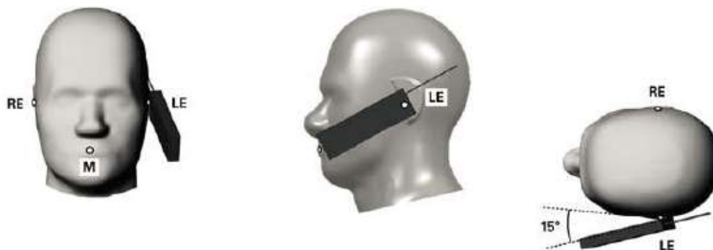
Fig.11.4 Illustration for Tilted Position
