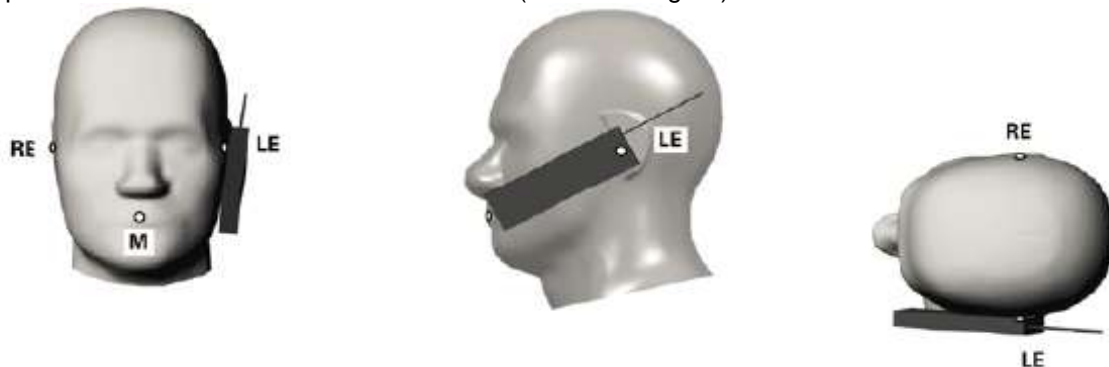
Fig. 11.3 Illustration for Cheek Position
