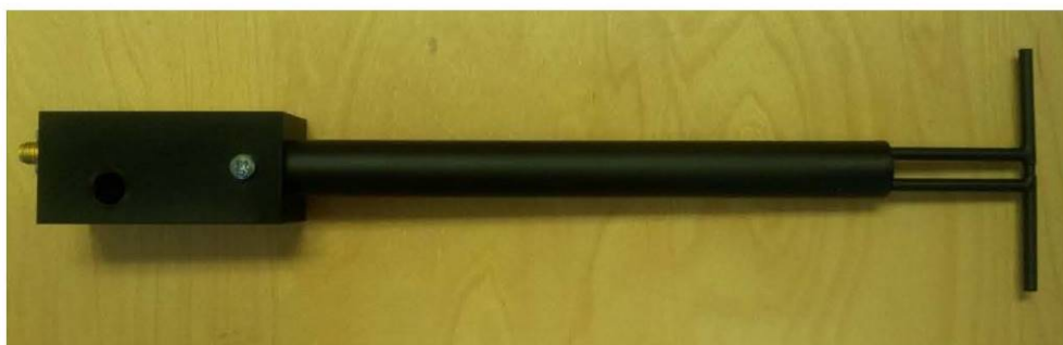
Figure 1 – MVG COMOSAR Validation Dipole
