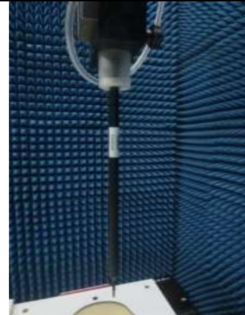
Fig.8.2 Photo of E-Field Probe
