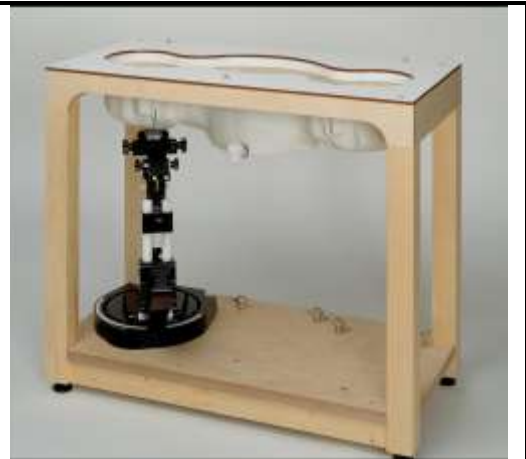
Fig. 8.7 Photo of SAM Twin Phantom
