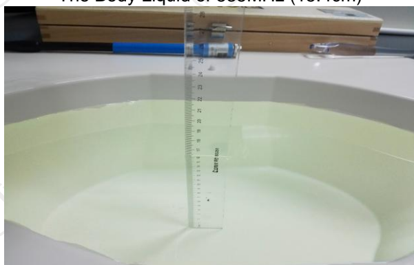
The Body Liquid of 1900MHz (16.4 cm)
