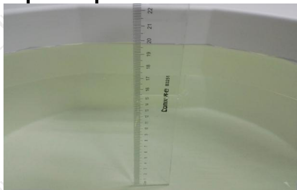
The Body Liquid of 835MHz (15.4cm)
