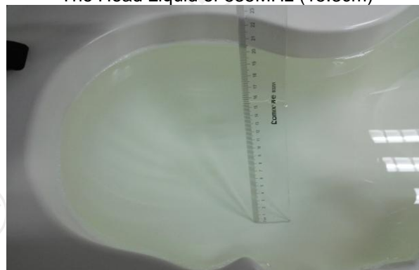
The Head Liquid of 1900MHz (15.5cm)
