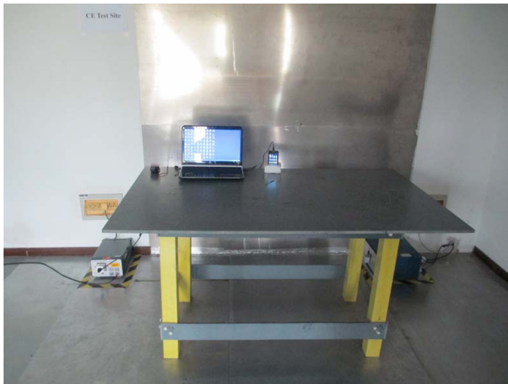
Conducted Emissions Test Setup Front View
