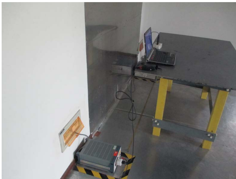
Conducted Emissions Test Setup Side View
