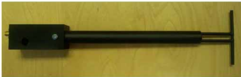
Figure 1 – MVG COMOSAR Validation Dipole
