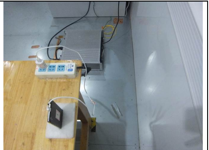
Conducted Emissions Test Setup Side View
