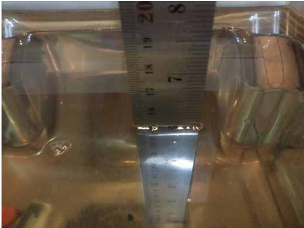
Liquid depth \geq 15\text{cm}
