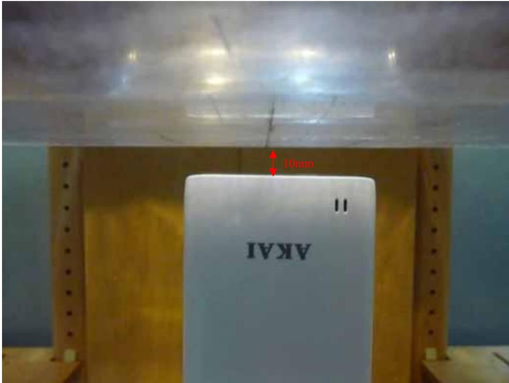
Body-worn Bottom Setup Photo (10mm)
