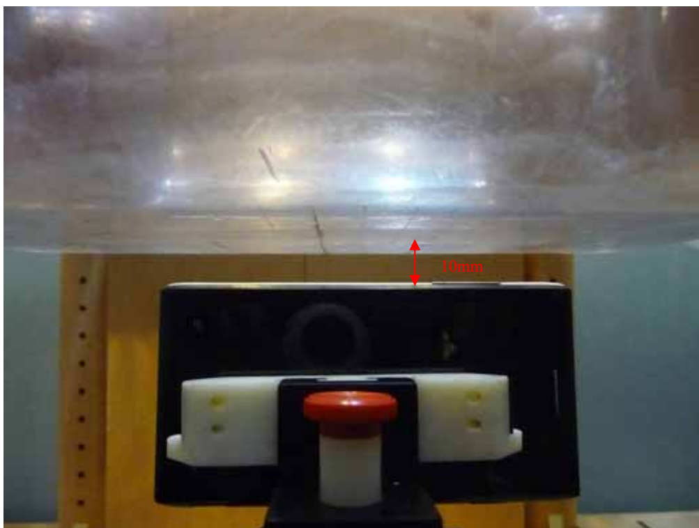
Body-worn Left Setup Photo (10mm)
