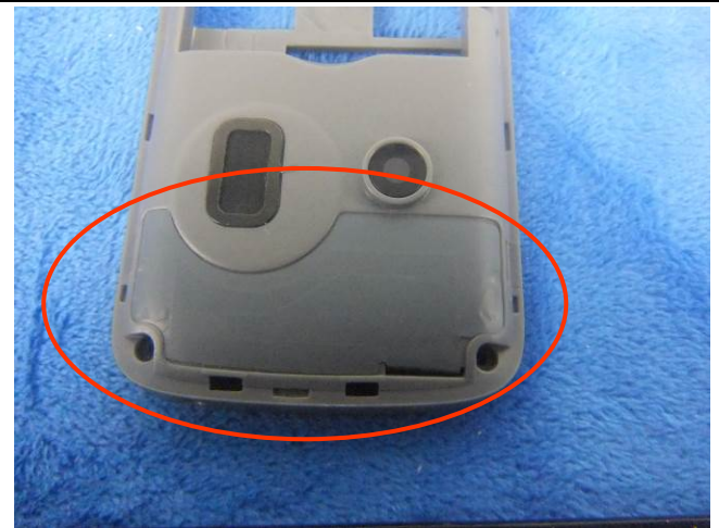
GSM/PCS/UMTS-FDD Antenna View
