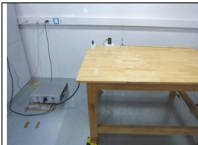
Conducted Emissions Test Setup Front View
