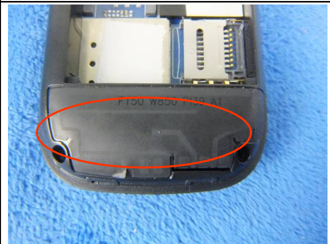
GSM/PCS/UMTS-FDD Antenna View
