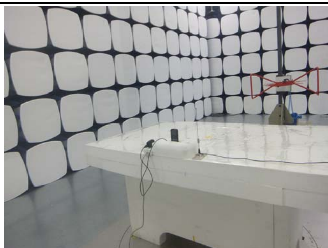
Conducted Emissions Test Setup Front View
