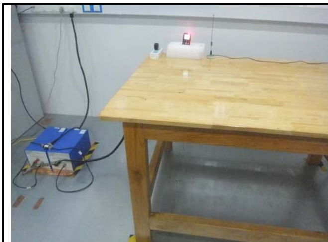
Conducted Emissions Test Setup Front View
