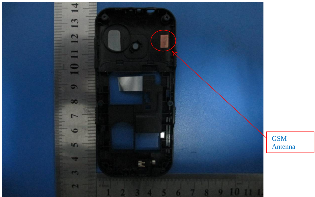
GSM Antenna Front View
