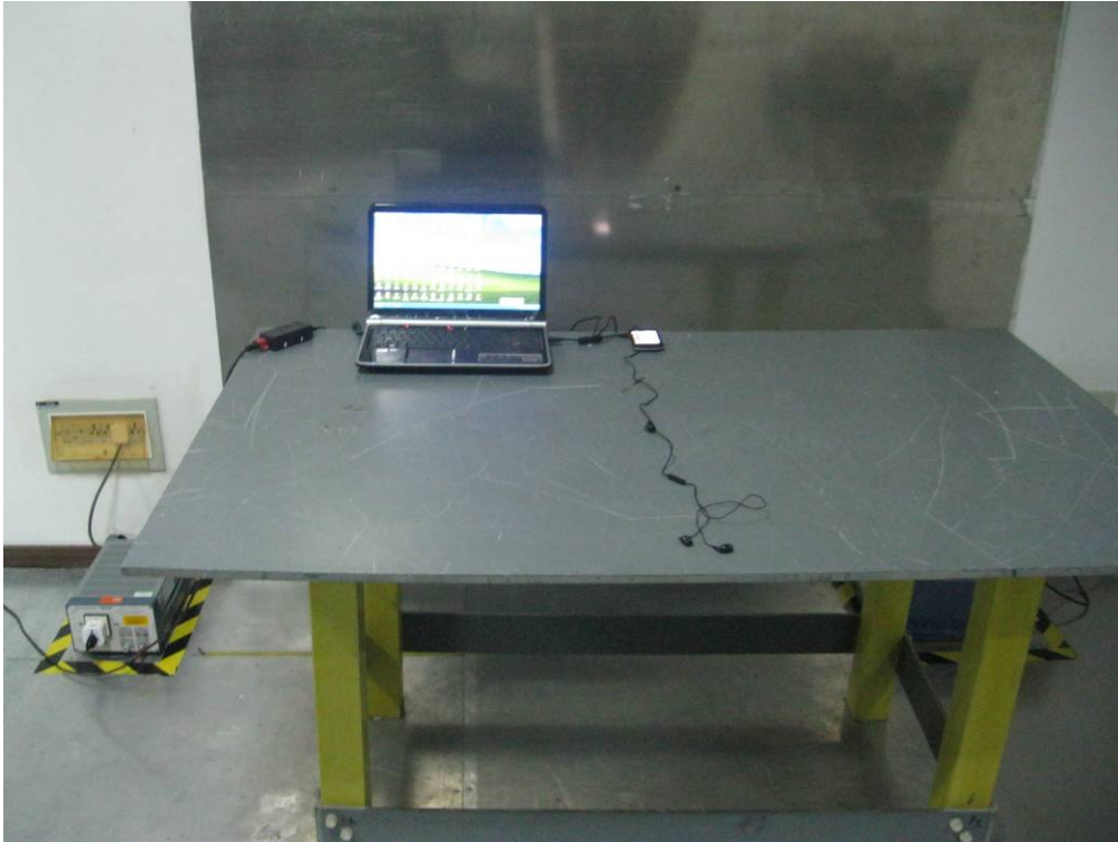
Conducted Emissions Test Setup Front View
