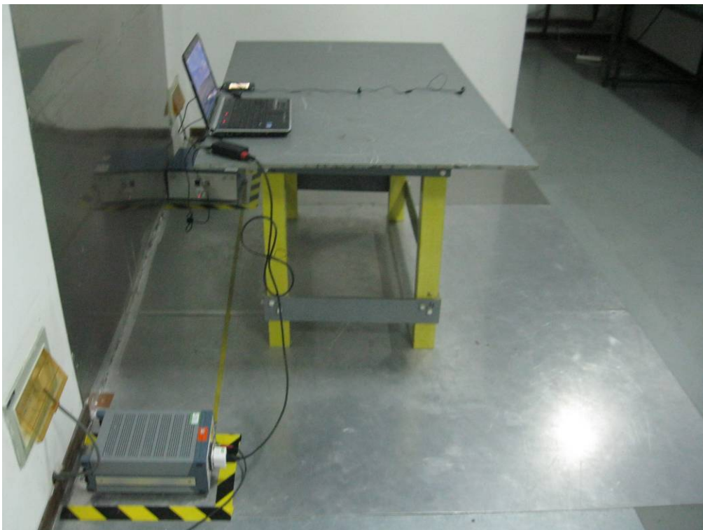
Conducted Emissions Test Setup Side View
